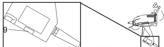
**MS 80 & MS 200:** The glue guns have a wire stand which is used to put down the applicator. Reka recommends folding in the wire stand when working with the applicator.
